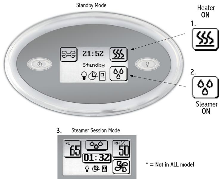
1. The heater can be switched on by pressing the heater icon in standby mode.
