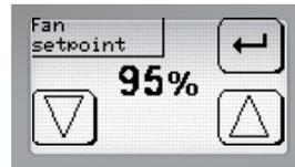
Press the fan icon (not in all models), to set the fan speed, in the range of 5% - 100%. After setting the preferred speed, user can go back to the previous menu with saved settings by waiting for 3 seconds to automatically return or pressing the enter button to return immediately.
