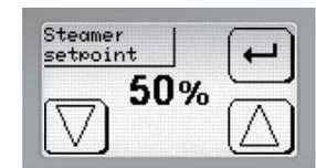
If no keys are pressed within 5 seconds after pressing the temperature button, the actual humidity in the sauna room is displayed again and changes are discarded.
