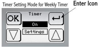
If "Off" is displayed weekly timer is not activated. Pressing Enter icon when off icon is chosen activates the timer and "On" is then displayed. Likewise push of Enter icon when "On" is chosen will inactivate the timer and "Off" will be displayed.
