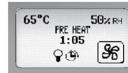
When the control unit turns the heater on upon pre-set time, pre-heat countdown mode will be displayed. Once the set Pre-heat time has finished, high tone can be heard and backlight in the display will be switched on to mark sauna is ready for use. Unit will go to Heater / Steamer On mode.
