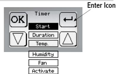
In "Timer" mode push of hammer icon open up settings display (see the picture). Choose the feature using arrow icons and press then enter to open up the setting display for that feature. Change parameters with arrow icons and confirm by pressing enter.
